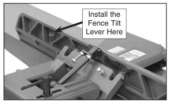
Figure 17. Tilt lever installation location.
